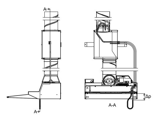
The exhaust air terminal (KSO-125) is locked in a way that it meets the requirements set for the smoke limiter (42 dm³/s @ 100 Pa). The exhaust air terminal must not be adjusted!
