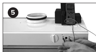
Measure the voltage from poles - and S, set speed 2 from potentiometer 2, etc.
