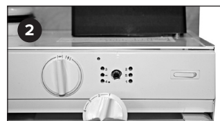
There are holes for adjustments and measurements underneath the knob
