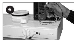
You may also carry out the measurement from the terminal block, at the places indicated by the wiring diagram.
