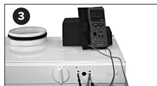
Measure the voltage from poles - and S, set e.g. speed 1 from potentiometer 1
