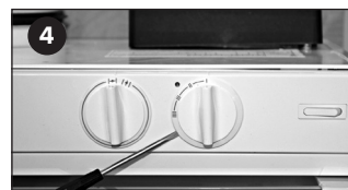
Replace the knob, set the ventilation control to the next speed, and remove the knob again.
