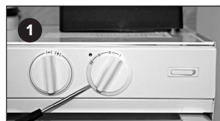
Set the ventilation control to position 1 and remove the knob by using a screwdriver, for example
