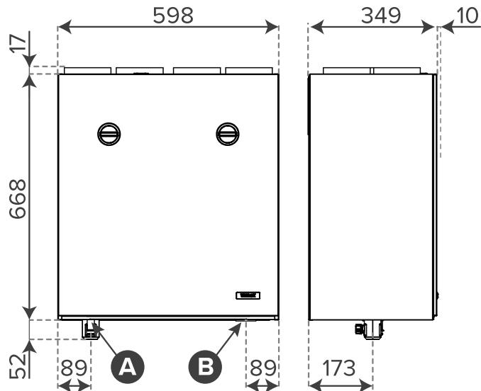
There are two condensing water discharge outlets at the bottom. The condensing water outlet or siphon is connected to a free, not plugged, discharge outlet.
