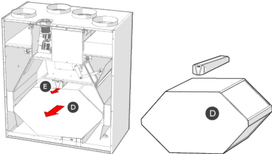
4. Lift and pull the cell (**D**) out of the unit.
