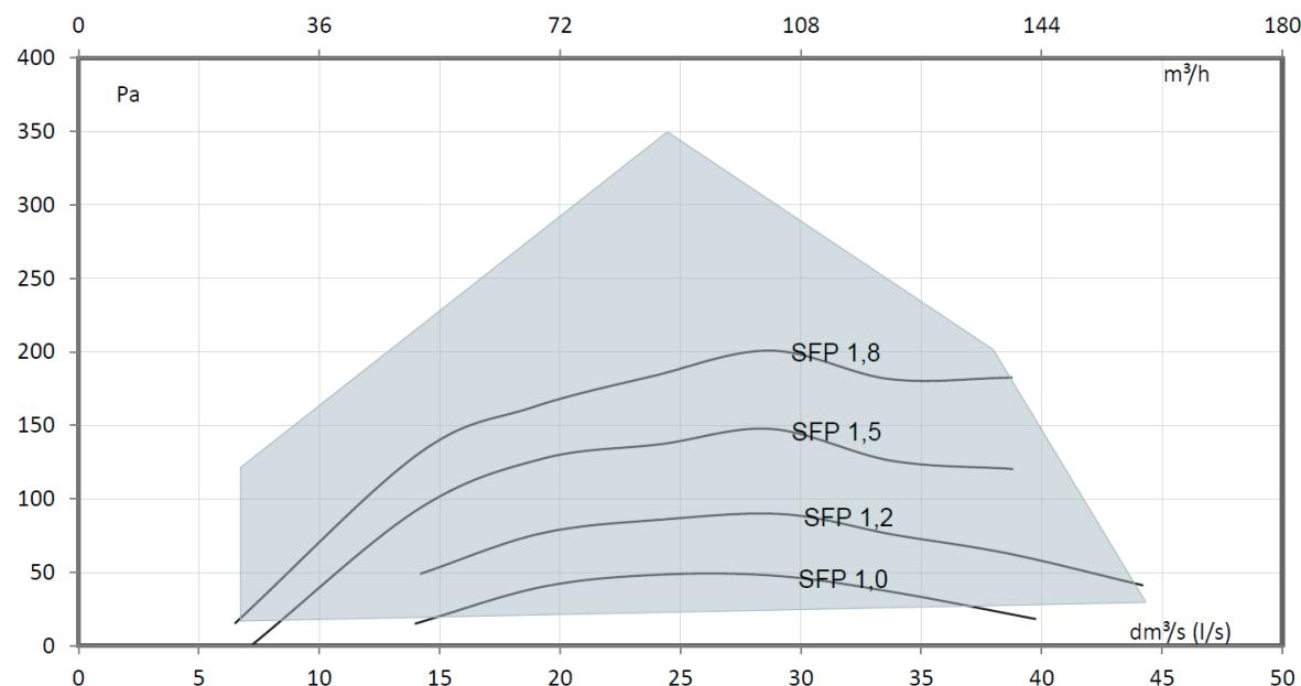
The recommended SFP (Specific Fan Power) rate is <1.8 (kW m<sup>3</sup>/s). At a lower total pressure, the SFP rate is lower.
