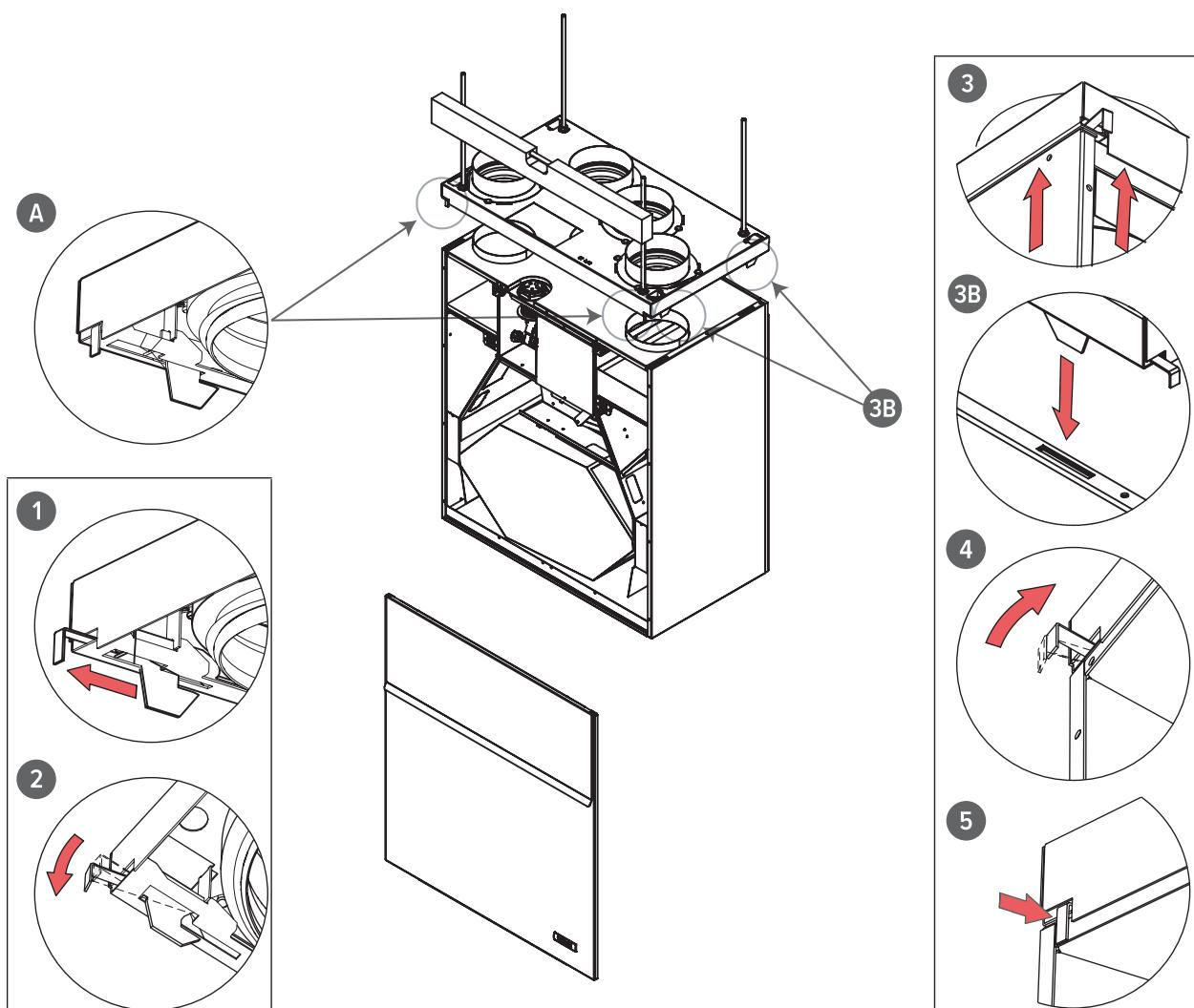
1. Fasten the M8 thread bars on the rafter frames or other frame structure and fasten the nuts onto the bars.
