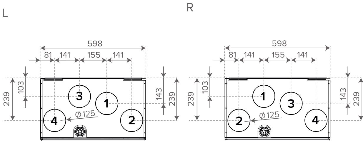
Inner diameter of the female collar  $\varnothing$  125 mm.
