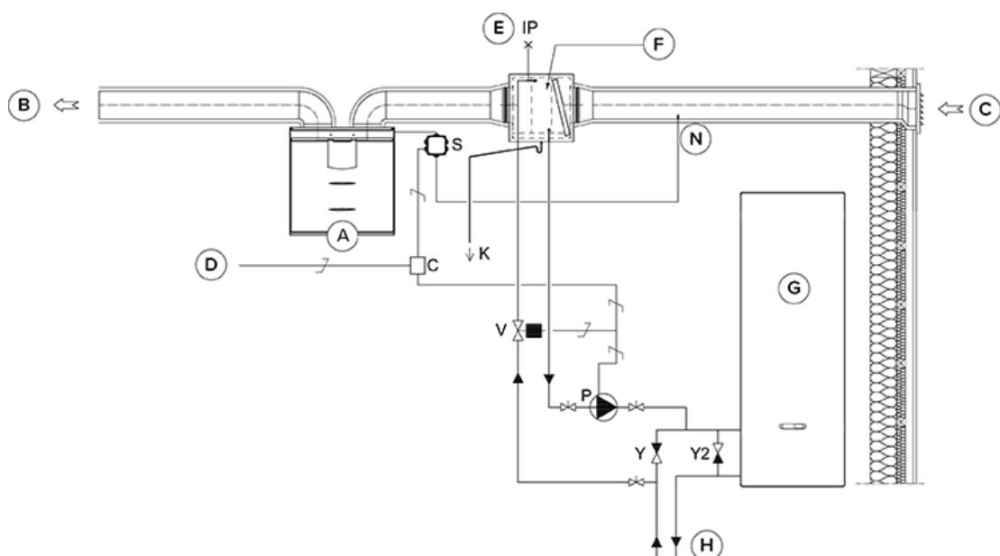
Figure 4. Duct radiator operation chart in the supply air duct
