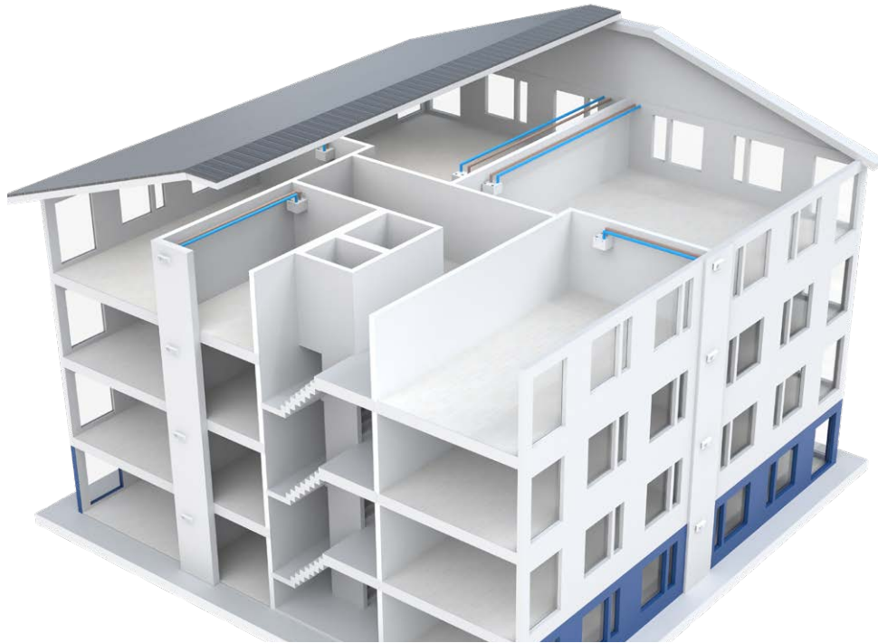
Alternative 1. An apartment-specific ventilation unit takes the outdoor air and removes exhaust air through the building's external wall, so there is no need for a duct running through the building to the roof.
