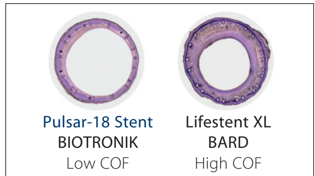
Figure 2. Preclinical results in a porcine model. The low-COF Pulsar-18 stent (Biotronik) caused less neointimal hyperplasia at 90 days compared to a high-COF stent.
