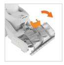
Lift the nozzle release clip and pull the nozzle forward to remove.
