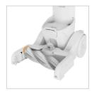
To replace the brushbars, align the right side of the first brushbar onto the circular gearing. Push the left tab downwards until it clicks into place. Repeat the same process with the other brushbar.
