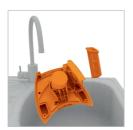
Rinse the filter and dirty water tank lid under warm water (max 40°C) to remove dirt/debris.
