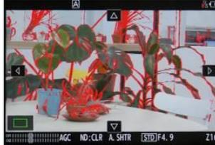
Adds colored highlights to in-focus edges. Highlight levels can be adjusted, and its color can also be selected from four different colors.
