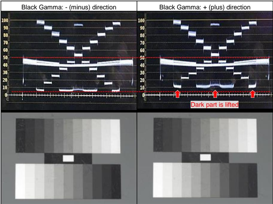
By utilizing Black gamma control, dark parts of the image such as hair lines, casted shadows etc. can be expressed without changing brightness of entire image.
