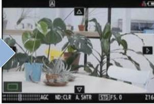
Part of image can be magnified up to 4 times (x2, x3, x4). Its magnification period can be set 3 different ways (see EXPAND MODE below).
