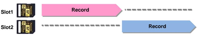
Note: The maximum continuous record time is up to 10 hours, recording stops when 10 hours has been reached. Recording will automatically recommence after a few seconds.
