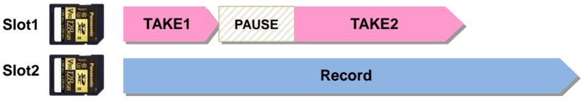
Note: To stop recording on slot2, keep pressing the USER button which has "BACKGR PAUSE" assigned to it or "EXIT" button for 5 seconds.
