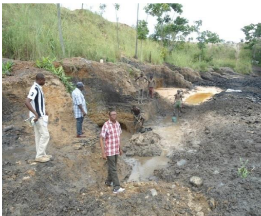
Fig. 3. Logging and sample collection at the Okaba coal field. Note the heavy acid minewaters within the mines
