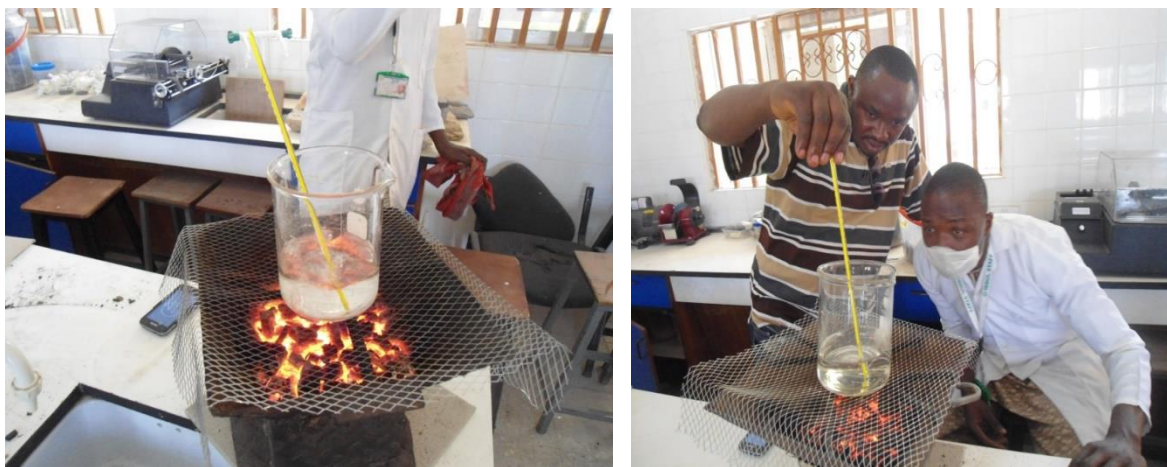
Fig. 8. Combustibility studies for the determination of the coal energy efficiencies and coalcombustion pathways by measuring the time it takes same quantity of each of the coaldeposits to bring same volume of water to boiling point as well as the temperature achieved at every 2 minutes using local cooking stove
