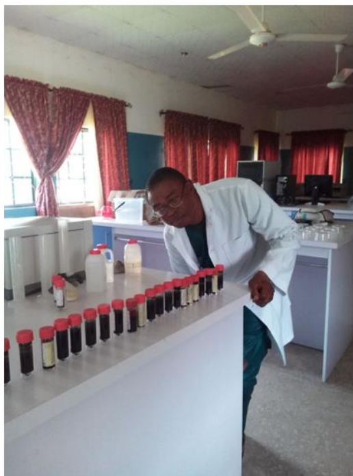
Fig. 11. Defusination experiment involved digestion of the pulverized coals with different types of organic acid and kept to react for 48 hours.
