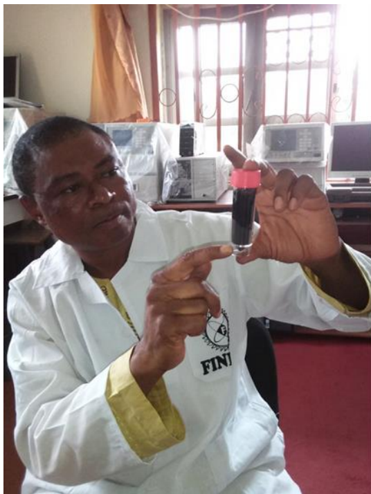
Fig. 11. Defusination experiment involved digestion of the pulverized coals with different types of organic acid and kept to react for 48 hours.
