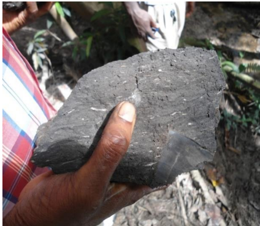
Fig. 4. Direct sample collection of coal in-situ at the Omelehu coal field
