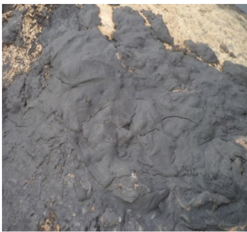
Fig. 7. In the absence of any coal exposure in Niger State, the team relied on the shaley coalsamples collected during the earlier study on Bida Basin hydrocarbons. These shaley coals are more suitable for oil and gas generation than for the production of smokeless fuel
