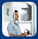
Patient's are held in a stable and comfortable position via the lateral positioning devices, handgrip and integrated chin rest
