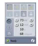
In manual mode user can adjust kV/mA values separately to reach maximum performance.
