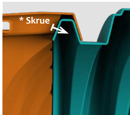
Overlap Endemodul og en stor ribbe.
