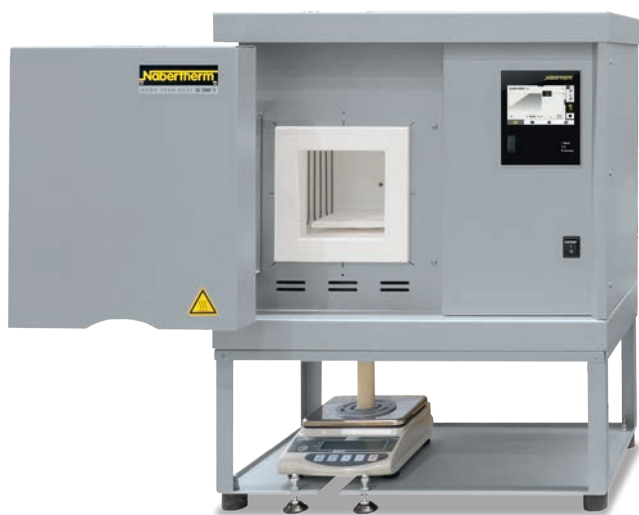
High-temperature furnace LHT 04/17 SW with scale for measuring weight reduction during annealing
