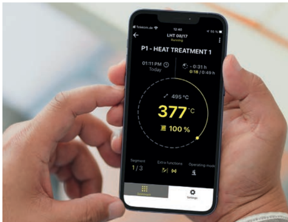
Display of program progress for each furnace
