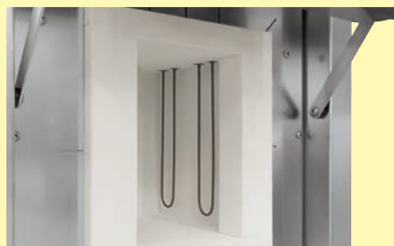
High-quality molybdenum disilicide heating elements
