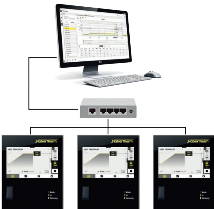
Example lay-out with 3 furnaces
