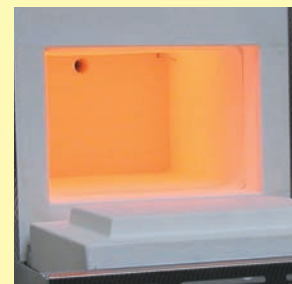
Muffle heated from four sides
