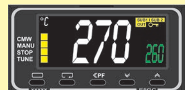
Example of an over-temperature limiter
