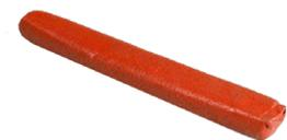
A one-part, ready-to-use, re-enterable, intumescent putty that can be easily formed to firestop through penetrations and blank openings in fire-rated assemblies.
