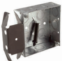
"UBS" Support Universal Back Side support to provide bracing on back of box for wall cavities 2-1/2" - 6" thick.
