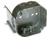
"J" Bracket Spurs, slotted holes for toe-nailing. Gauging notches at 3/8" and 1/2".
