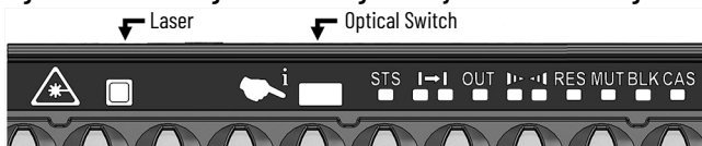
Figure 9 - Use the Integrated Laser Alignment System for Positioning
