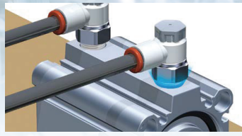
Leakage from piping connection due to aging
