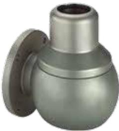
Wall Joint with vertical socket for mounting to vertical surfaces. Cover to facilitate wiring. Turns through 340 degrees with rotation limiter. Preset torque. Maintenance-free bearings. Type 304 polished stainless steel finish. Includes gaskets. Wall-mounting fasteners not provided.
