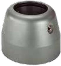
Flange coupling for attaching enclosures. Turns through 340 degrees with rotation limiter. Preset torque. Maintenance-free bearings. Type 304 polished stainless steel finish. Includes gaskets and mounting hardware.
