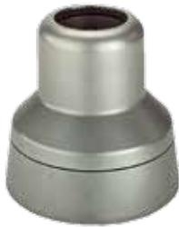
Swivel Base for mounting to machine or floor. Turns through 340 degrees with rotation limiter. Preset torque. Maintenance-free bearings. Type 304 polished stainless steel finish. Includes gaskets. Base-mounting fasteners not provided.
