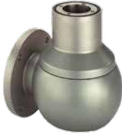
Swivel Wall Coupling for direct mounting of enclosure to vertical machine surfaces. Turns through 340 degrees with rotation limiter. Cover to facilitate wiring. Preset torque. Maintenance-free bearings. Type 304 polished stainless steel finish. Includes gaskets and enclosure mounting hardware. Wall-mounting fasteners not provided.
