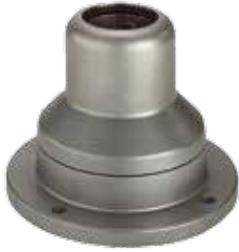
Swivel Base for mounting to machine or floor. Turns through 340 degrees with rotation limiter. Preset torque. Maintenance-free bearings. Type 304 polished stainless steel finish. Includes gaskets. Base-mounting fasteners not provided.
