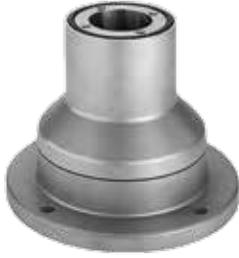
Swivel Base External Bracket Coupling for mounting enclosures directly to a machine or the floor. Turns through 340 degrees with rotation limiter. Preset torque. Maintenance-free bearings. Type 304 polished stainless steel finish. Includes gaskets and enclosure mounting hardware. Base-mounting fasteners not provided.
