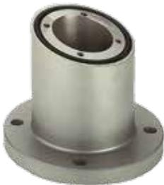
Rigid 15-degree coupling for direct mounting of enclosures to horizontal and vertical surfaces. Type 304 polished stainless steel finish. Includes gaskets and enclosure mounting hardware. Base-mounting fasteners not provided.
