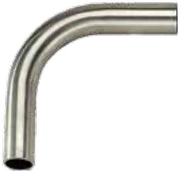
L-Shaped Tubing has an outer diameter of 48.3 mm (1.90 in.) and is made from 3.6-mm-thick Type 304 polished stainless steel. It is used with coupling sleeves and straight tubing to provide the desired system configuration.
