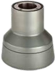
Swivel Base Internal Bracket Coupling for directly mounting enclosures to a machine or the floor. Turns through 340 degrees with rotation limiter. Preset torque. Maintenance-free bearings. Type 304 polished stainless steel finish. Includes gaskets and enclosure mounting hardware. Base-mounting fasteners not provided.
