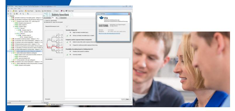
SISTEMA is a FREE software tool designed by Germany's BGIA (Institute for Occupational Safety & Health) to evaluate the Performance Level (PL) of a safety function using ISO 13849-1. A key part of a safety system is verifying that the solution meets the safety performance level of the hazard.
