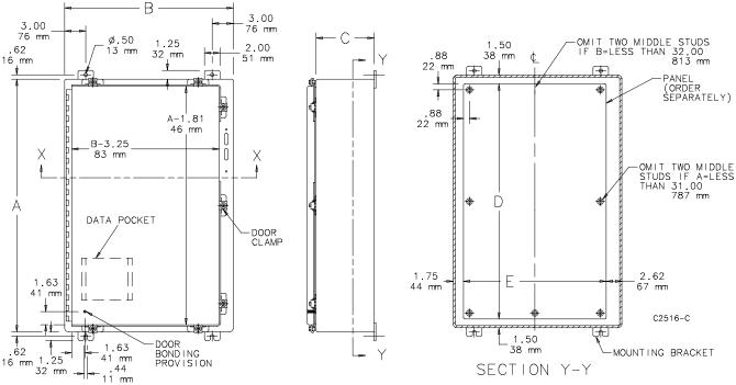
NOTE: 1. 12 gauge panels have flanges along two sides when the side dimension is more than 21.00 inches (533mm). Panels A24P20 and A24P24 have flanges on four sides.
