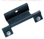
Optional hinging for steel solid, window or disconnect doors. The 180-degree hinges provide a door opening up to 260-degrees on single-bay enclosures. These hinges mount to the door flange and have a low-profile appearance. The kit includes three hinges with textured black polyester powder paint and all necessary mounting hardware. Cannot be used on ProLine FloTek or ConneckTel front doors.
