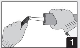
Cartridge: Cut off tip of nozzle to desired size. Sausage Pack: Cut off tip of nozzle to desired size, cut and remove foil crimp on one end of sausage pack. Pail: Remove lid.
