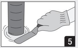
Tool sealant to be flush with substrate.
