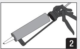
**Cartridge:** Insert cartridge into cartridge applicator.
