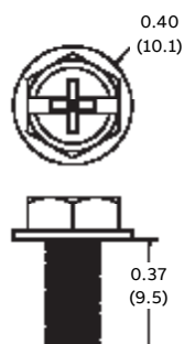
#10–32 Combination Phillips, slotted and 3/16 hex washer head
