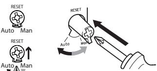
**en** In case of adjusting "RESET Auto", which means automatic reset after tripping, the motor may restart automatically. This automatic restart could injure persons and damage material.
