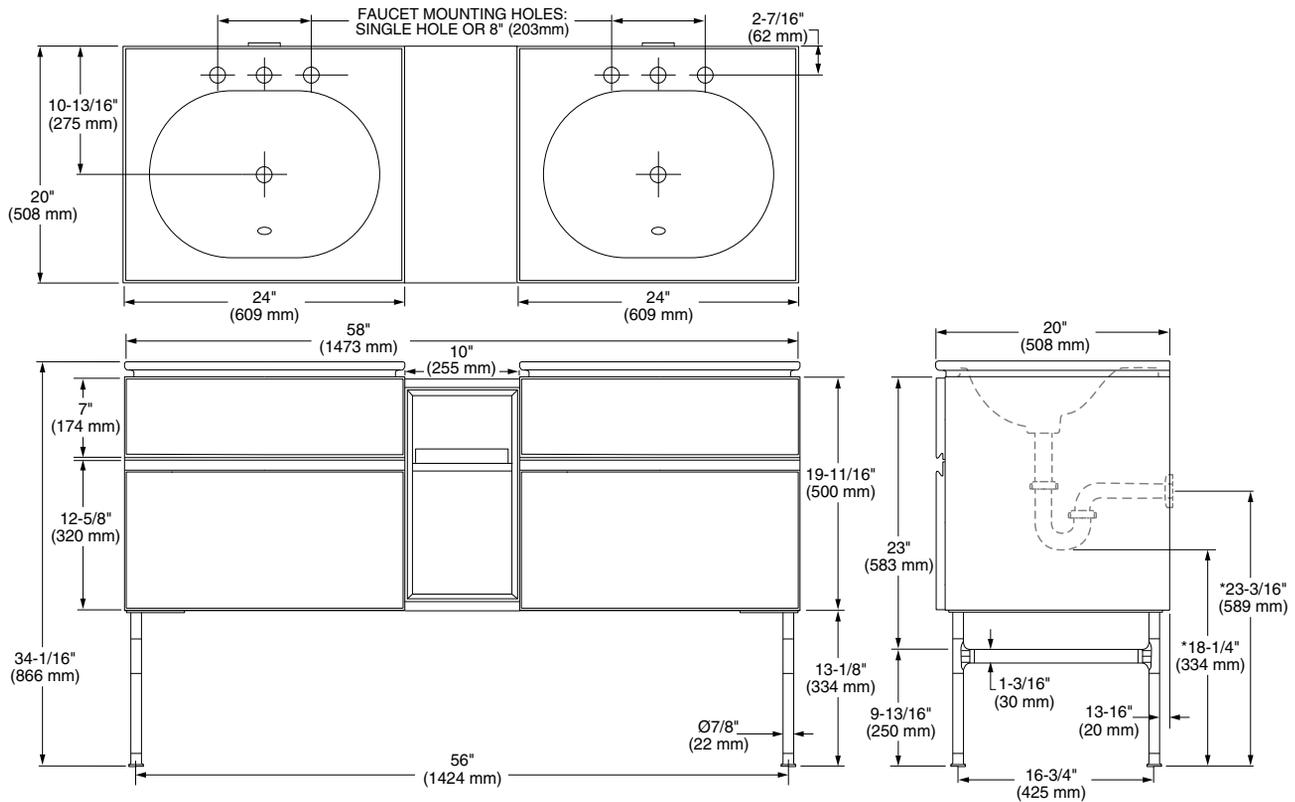
**NOTE:** Vanities can be installed with optional vanity leg set shown or mounted directly to wall.
