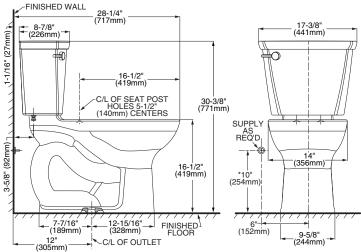
THIS TOILET IS DESIGNED TO ROUGH-IN AT A MINIMUM DIMENSION OF 305MM (12") FROM FINISHED WALL TO C/L OF OUTLET.
