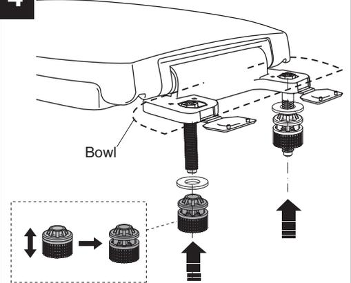
When opened, nuts can slip over threads for rapid installation.
