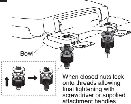
When closed nuts lock onto threads allowing final tightening with screwdriver or supplied attachment handles.
