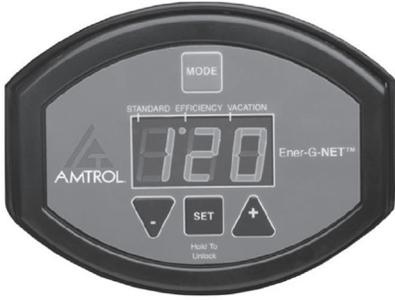
Ener-G-NET incorporates all of the temperature sensing and control necessary for HYDROMAX® operation. Built-in switching relays may be wired to operate the boiler control and circulator pump or zone valve. The diagram below illustrates these internal switching functions.
