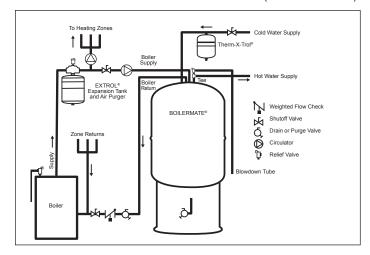
PIPING USING ZONE VALVE WITH EXISTING HEATING SYSTEM CIRCULATOR
