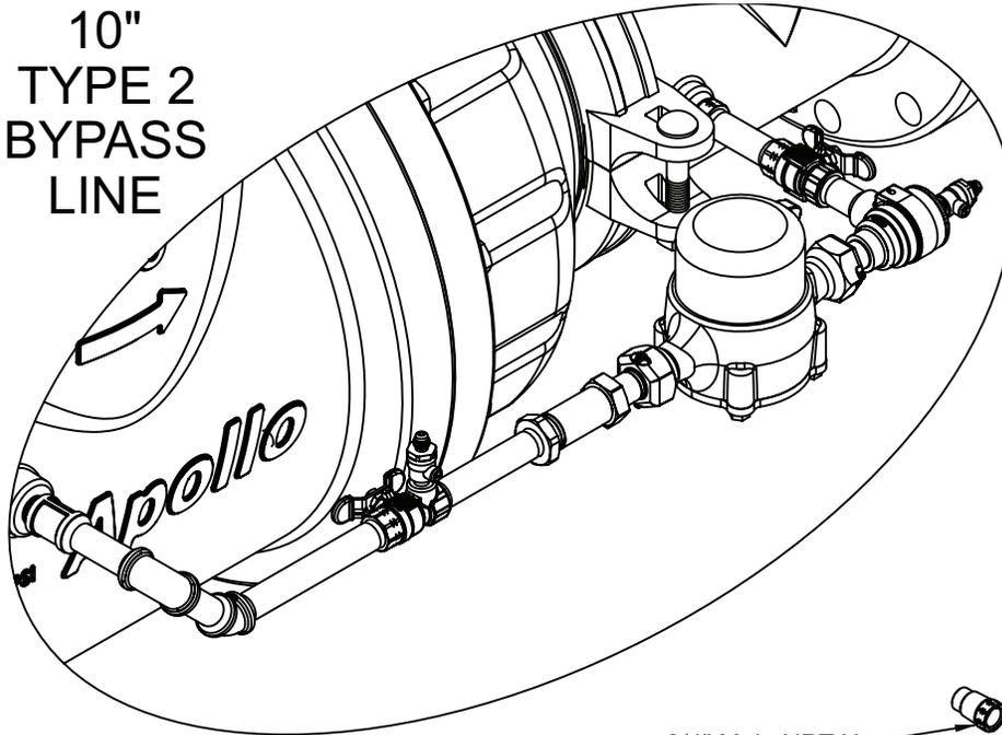
APPLY TEFLON TAPE TO PIPE THREADS AND INSTALL COMPONENTS AS SHOWN.
