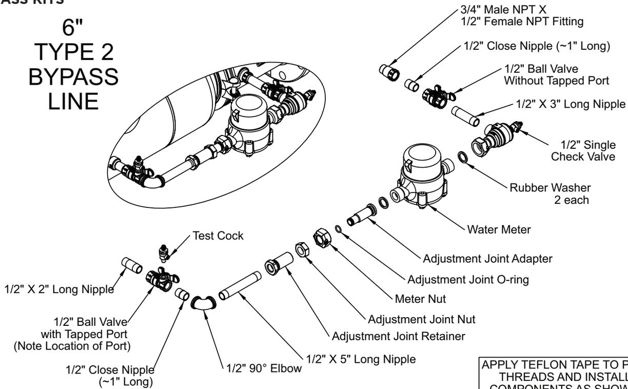
APPLY TEFLON TAPE TO PIPE THREADS AND INSTALL COMPONENTS AS SHOWN.
