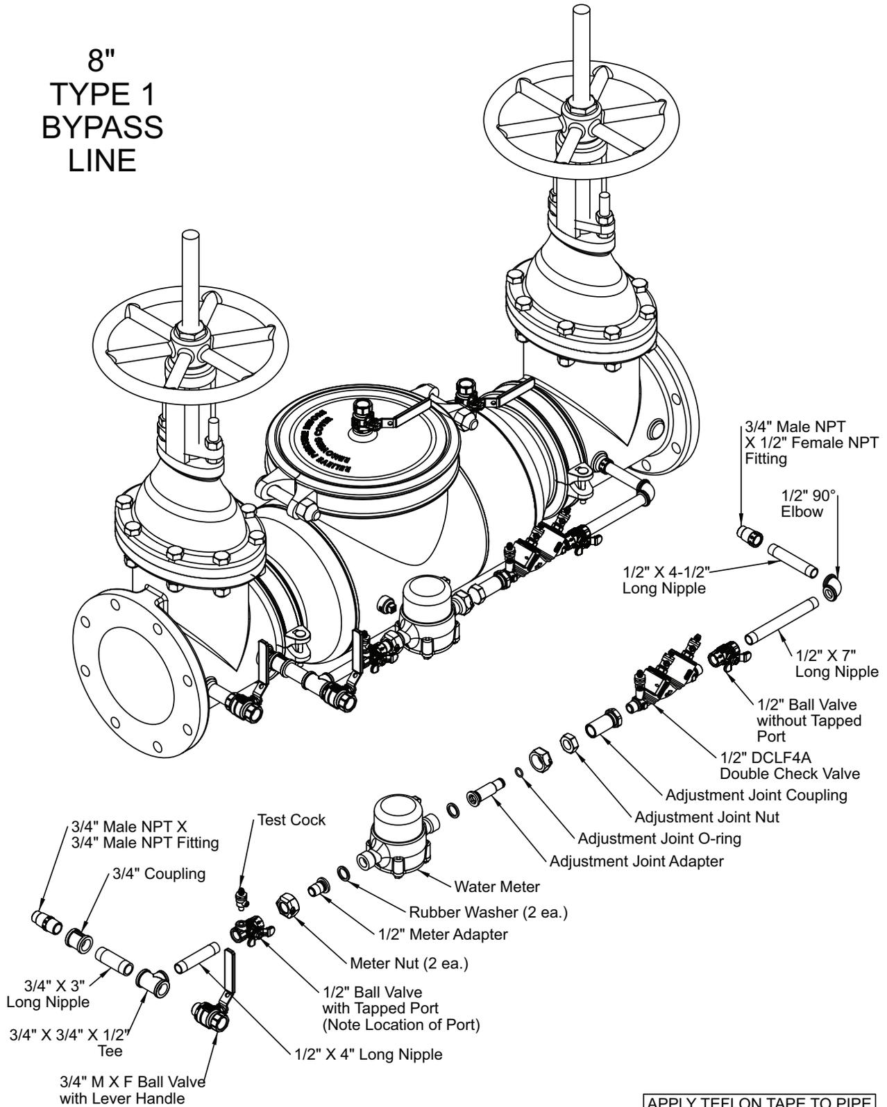
APPLY TEFLON TAPE TO PIPE THREADS AND INSTALL COMPONENTS AS SHOWN.
