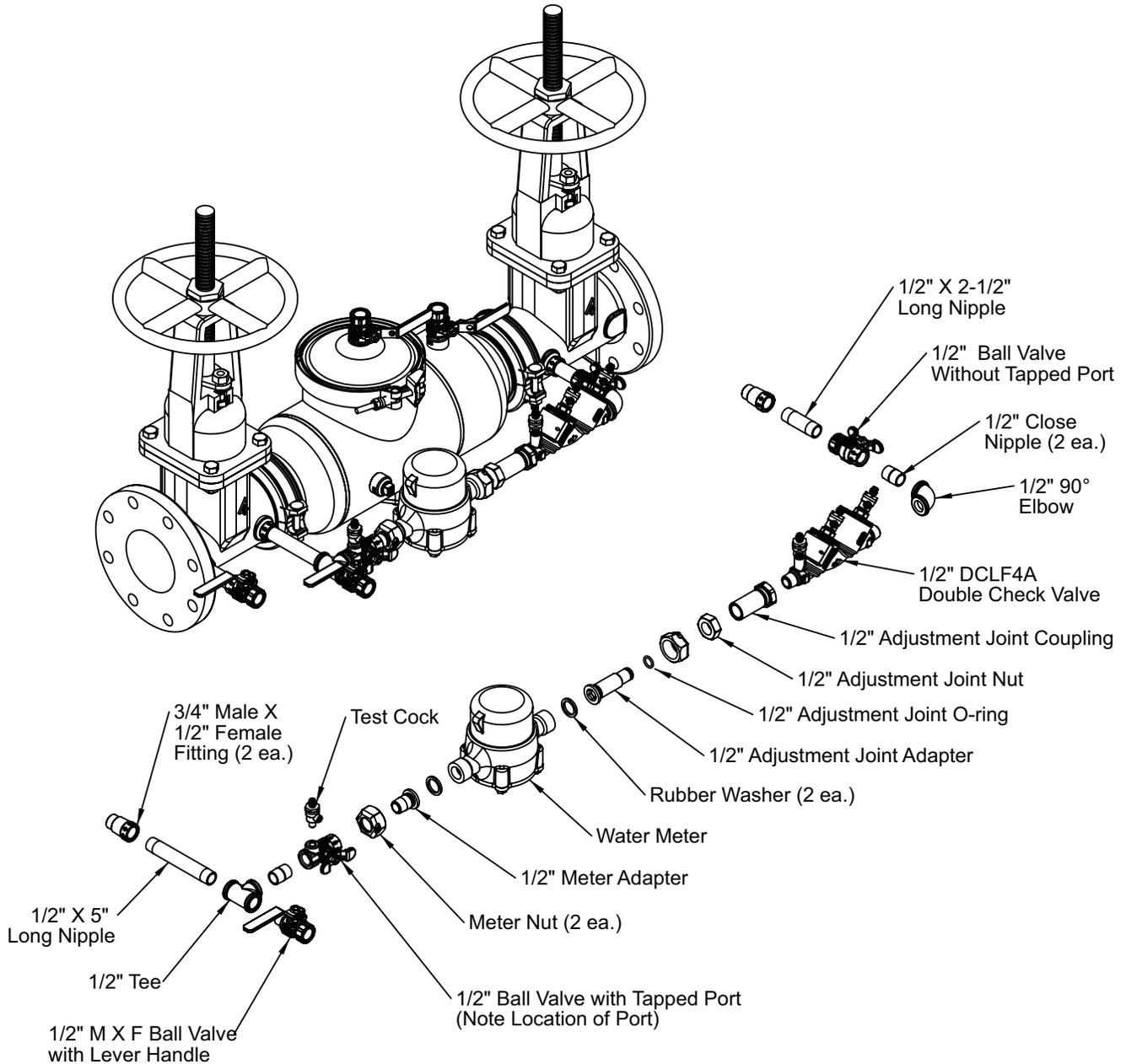
**APPLY TEFLON TAPE TO PIPE THREADS AND INSTALL COMPONENTS AS SHOWN.**
