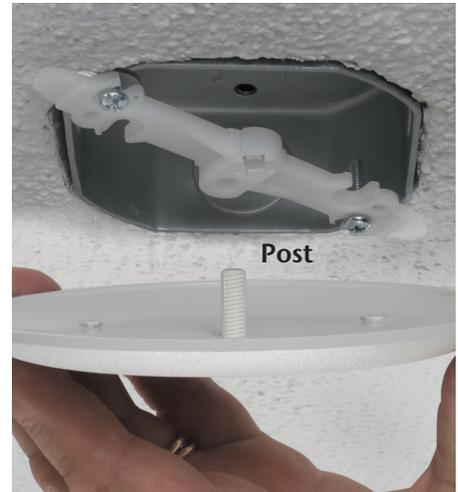
**3** On flat ceilings, push threaded post into the 'A' opening to seat the cover. On textured or uneven ceilings, thread the post into the 'B' opening until tight.
