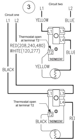
**Sequence of Operation- Double Element, Non-Simultaneous Operation, 3 Phase.**
