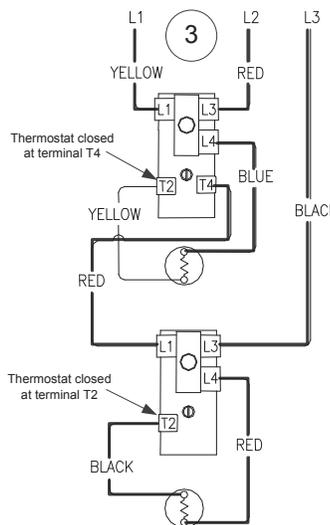
4 When the lower thermostat is satisfied, it opens at terminal T2 interrupting the current flow through the lower element. The system is now in stand-by mode waiting for the next call for heat.
