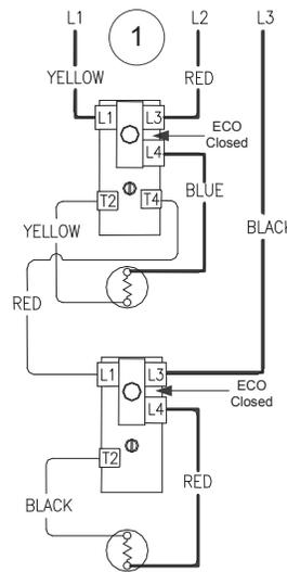
2 Tank is cold therefore both thermostats are closed at terminal T2 (calling for heat). The circuit is complete through the upper thermostat only allowing current to flow through the upper element.
