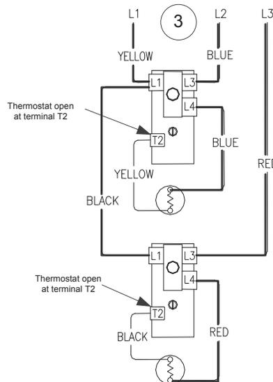
Some electric utility companies will offer discounts for using electricity during “Off Peak” Times of the day. The system allows the use of an “Off Peak” meter, which interrupts power to the lower element during high power demand periods.
