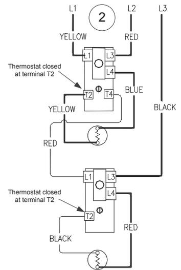
3 When the upper thermostat is satisfied, it opens at terminal T2 interrupting current flow through upper element, and closes at terminal T4 allowing voltage to pass to terminal L1 of lower thermostat. This completes the circuit through the lower thermostat allowing current flow through lower element.
