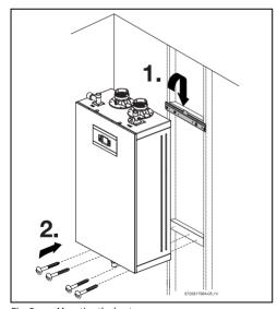
Fig. 9 Mounting the heater
