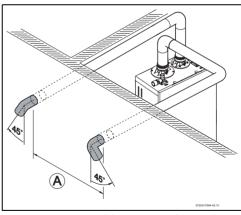
Fig. 14 Horizontal parallel venting system (twin pipe)
