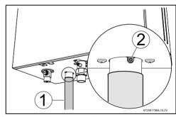
Fig. 20 Appliance drain installation
