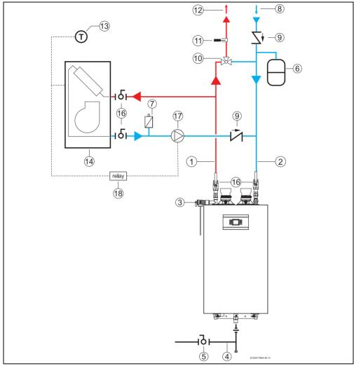
Fig. 34 Hydro air system with water heater
