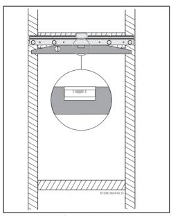
Fig. 8 Leveling wall mounting bracket
