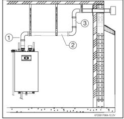
Fig. 23 Installation Recommendation for Placement of Backdraft reducer
