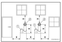
Fig. 17 Vent and combustion air pipe position of a sealed combustion system
