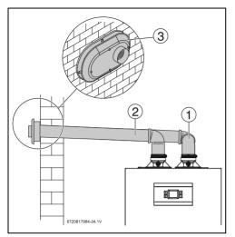
Fig. 18 Horizontal venting system (sealed combustion)
