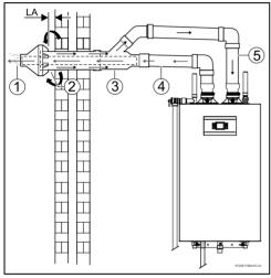
Fig. 12 Horizontal venting system (concentric vent)
