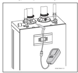
Fig. 62 CO<sub>2</sub> measuring port
