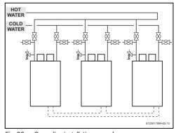
Fig. 33 Cascading installation example
