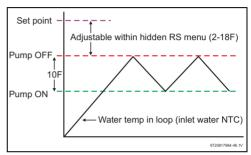
Fig. 31 Pump activation and deactivation thresholds
