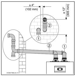
Fig. 16 Horizontal venting system (sealed combustion)
