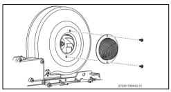
Fig. 54 Remove/assembly air filter
