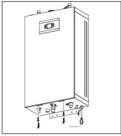
Fig. 3 Loosen two Phillips head screws
