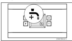
Fig. 57 Combustion Auto Adjust - Open Taps
