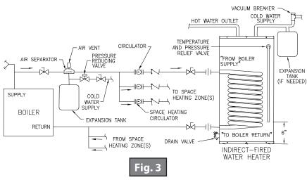
**Water Boiler Piping with Circulators**
