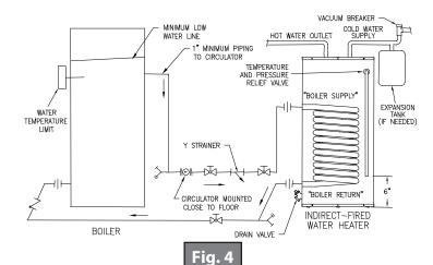
Typical Steam Boiler Connections (connections available below the water line)
