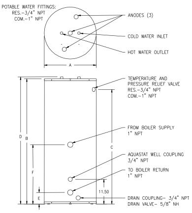
Figure 1 - Tank Layout
