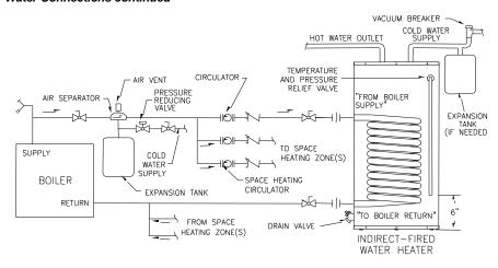
Figure 3 - Water Boiler Piping with Circulators
