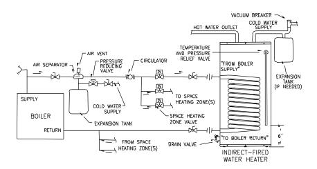
Figure 2 - Water Boiler Piping with Zone Valves
