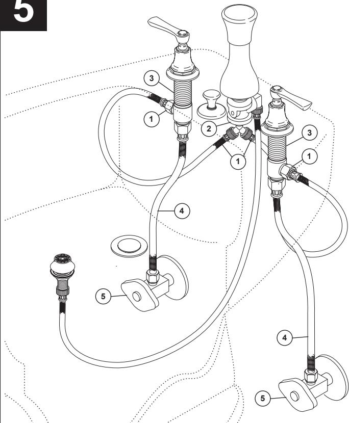
Connect 12" hoses (1) from "Y" on diverter valve (2) to outlets on hot & cold end valve bodies (3) as shown. Tighten firmly but do not over tighten. Connect inlet hoses (4) to hot and cold valve inlets (5) as shown. Tighten firmly but do not over tighten.
