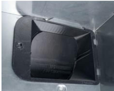
EzDuct™ Connector enables room-side installation without attic access. Attach the housing, pull the duct through, attach the EzDuct™ Connector and reset it with one screw.
