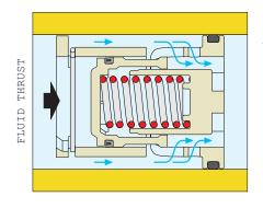
If the differential pressure is within the control FLOW RATE range, the spring-loaded piston is positioned to give the fluid a free flow area permiting regular flow at the **nominal rate** for which the FlowCal<sup>™</sup> is set up.
