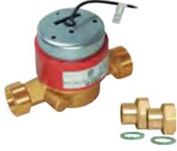
Single jet rotary pulse flow meter measures liquid flow for energy heat metering production or consumption. Accurate to International Standards OIML R75, EN1434 and MID.
