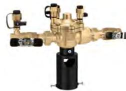
Testable reduced pressure zone backflow preventer. DZR low lead brass body. Max. working pressure: 150 psi. Max. working temperature: 150°F. Certified to: ASSE 1013, CSA B64.4, NSF372, Low Lead Laws and listed by ICC-ES. Meets codes IPC, IRC & UPC for use in accordance with the U.S. and Canadian plumbing codes.
