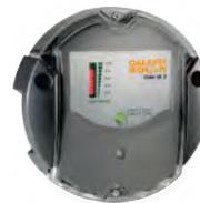
*iSolar*<sup>™</sup> DL2 intelligent web enabled datalogger connects to VBus data terminals on one *iSolar*<sup>™</sup> controller. VBus input terminals: 1. Ethernet connection: RJ45 socket. Integrated SD slot: 1. Ambient temperature: 32—100°F. Input voltage: 5 VDC ±5%. Power voltage adapter: 100—240 V. Max. current: 350 mA.
