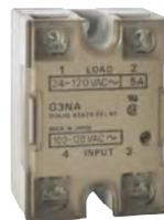
SSRs (Solid State Relays) is an isolation speed control relay which will speed control up to a 5 Amp solar pump based on the output speed control voltage of the *iSolar* solar controllers.
