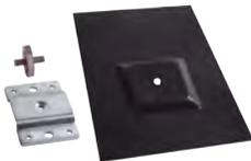
Flashing kit with 3/8" stud for attaching U mounts and other brackets using the supplied 3/8" stainless steel nut & washer. Black painted aluminum 6061 T6 flashing 14¾"L x 9½"W x 0.6"H, galvanized steel base plate with six mounting holes and double stud.
