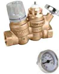
Adjustable thermal balancing valve for domestic hot water recirculation circuits. With by-pass valve for thermal disinfection with optional 656 actuator. Drywell for temperature gauge. DZR low-lead brass body. Optional outlet check valve Max. working pressure: 230 psi Adjustment temperature range: 95°F — 140°F Cv max: 2.1; Cv min: 0.23 Cv disinfection: 1.2; Cv design: 0.52 Certified to Low Lead Laws and listed by ICC-ES for use in accordance with the U.S. and Canadian plumbing codes.
