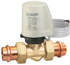
Two-way thermo-electric zone valve. Complete with 656414 actuator. Spring return. Normally closed. Brass valve body and trim. Max. body pressure: 150 psi. Max. Temperature: 200°F. Max: ΔP close-off pressure: 20 psi. Power supply: 24 V AC/DC. Initial current draw: ≤ 250 mA. Power consumption: holding: 3 W inrush: 6 VA Rating of micro-switch contacts: 5 A (24 V). 31.5" wire lead connection.
