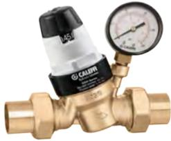
Pre-adjustable pressure reducing valve for residential and commercial applications. DZR low lead "Ecobrass" body. Unique noise reducing pressure balanced cartridge. Low friction anti-scale moving parts. High flow seat design. Dial indicator with direct readout. Replaceable cartridge. Integral stainless steel filter. Adjustment locking screw.
