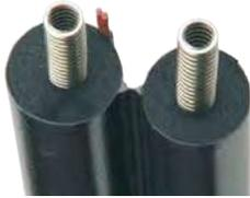
SolarFlex™ stainless steel piping with EPDM insulation. Used to connect solar collector with storage tank. Integrated sensor cable saves time and reduces cost. Packaged in a 50 foot continuous coil ensures a leak-free installation. Max. working pressure: 150 psi. Max. fluid temperature: 350°F. Min. surface temperature: -60°F. Min. bend radius: 5". Flammability: Class VO. Flame spread/smoke density: 25/50. Agency approvals: ASTM D 635 ASTM C 177
