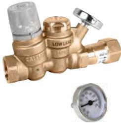
Adjustable thermal balancing valve for domestic hot water recirculation circuits. Drywell for temperature gauge or probe. DZR low-lead brass body. Optional check valve. Optional outlet temperature gauge. Max. working pressure: 230 psi Adjustment temperature range: 95°F — 140°F Cv max: 2.1; Cv min: 0.23; Cv design: 0.52 Certified to Low Lead Laws and listed by ICC-ES for use in accordance with the U.S. and Canadian plumbing codes.
