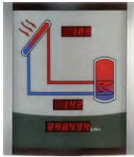
Smart display SD3 connected to VBus data interface is used for displaying data from *iSolar*<sup>™</sup> controller; collector temperature, storage temperature and total energy heat produced. An additional power supply is not required. Bright LED displays. Power supply: via VBus. Mounting: wall.
