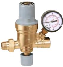
Pre-adjustable automatic filling valve, anti-scale, visual system pressure indicator. Complete with manual shut-off valve, strainer and check valve. Brass body.
