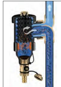
The dirt separator with magnet combines the action of the internal element and magnet. The impurities in the water strike the internal element and are separated, dropping into the bottom of the body where they are collected.
