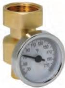
Point of distribution mixed temperature gauge adaptor fits 1" male union thread mixing valves. Removable gauge fits into pocket well. Gauge scale: 30–210°F. Gauge accuracy: ± 6°F. Gauge dial: 2" diameter. Certified: Low-lead brass.
