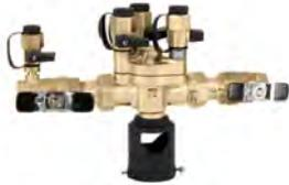
Testable reduced pressure zone backflow preventer. DZR low lead brass body. Max. working pressure: 150 psi. Max. working temperature: 150°F. Certified to: ASSE 1013, CSA B64.4, NSF372, Low Lead Laws and listed by ICC-ES. Meets codes IPC, IRC & UPC for use in accordance with the U.S. and Canadian plumbing codes.
