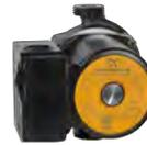
Replacement single speed 120 V, 1" male union thread. Flow 36 feet head / 8 gpm. Agency approval: cULus. (install in-line with NA122 union fittings on page 84)
