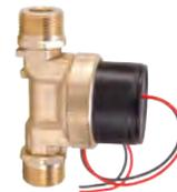
8 to 34 VDC, DC Strong solar pump for mounting in solar stations. 15 feet head / 7 gpm at 24 VDC. 8 feet head / 4 gpm at 12 VDC. Power consumption: 30—45 W. Max. working pressure: 150 psi. Max. temperature: -10—230°F.
