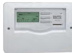
*iSolar*<sup>™</sup> DL3 intelligent web enabled datalogger / BACnet IP gateway connects to VBus data terminals on six *iSolar*<sup>™</sup> controllers. VBus input terminals: 6. Pt1000 sensor inputs: 3. Current loop input: 4—20 mA. Ambient temperature: 32—100°F. Input voltage: 12 VDC ±5%. Power voltage adapter: 100—240 V. Max. current: 1 A. Ethernet connection: RJ45 socket. USB connection: 1. Integrated SD card: 1 slot.
