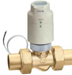
Two-way thermo-electric zone valve. Complete with TwisTop™ (code 656354) actuator. Spring return. Normally closed. Brass valve body and trim. Max. body pressure: 150 psi. Max. Temperature: 200°F. Max: ΔP close-off pressure: 20 psi. Power supply: 24 V AC/DC. Initial current draw: ≤ 250 mA. Power consumption: holding: 3 W inrush: 6 VA Rating of micro-switch contacts: 5 A (24 V). 31.5" wire lead connection.
