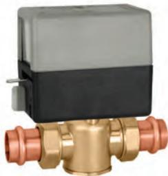
Two-way zone valve. Spring return. Normally closed actuator. Auxiliary micro-switch. Max. body pressure: 300 psi. Overall length: 5-5/8". Temperature range: 32–240°F. Suitable fluids: water, 50% max. glycol, 15 psi max steam. Power supply: 24 V AC. Power consumption: 5 W, 7 VA. Rating of auxiliary micro-switch contacts: 0.0 A min, 0.4 A max 24 V (24 V only). UL873, cULus Listed & CE. UL 1995 sec. 18 air plenums and ducts. US Patent 7,048,251.
