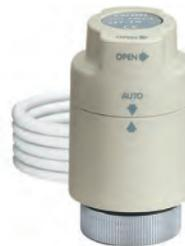
TwisTop™ thermo-electric actuator for use with 1163xx Series. Twist the top to manually open. Power supply: 24 V AC/DC. Initial current draw: ≤ 250 mA. Power consumption: 3 W. Rating of micro-switch contacts: 5 A (24 V). 31.5" wire lead connection. US Patent 7,617,989 B2.
