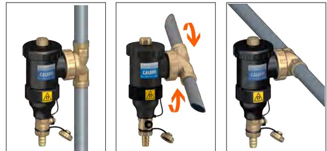
The special coupling between the locking nut and the mounting base allows the DIRTMAG® dirt separator to be rotated for installation to either vertical or horizontal pipes, while maintaining the same operating performance.
