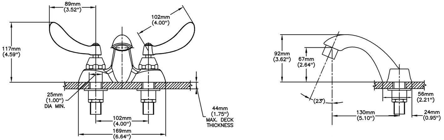
INLETS: 1/2" MIP/COUPLING NUTS (NUTS NOT SUPPLIED)
