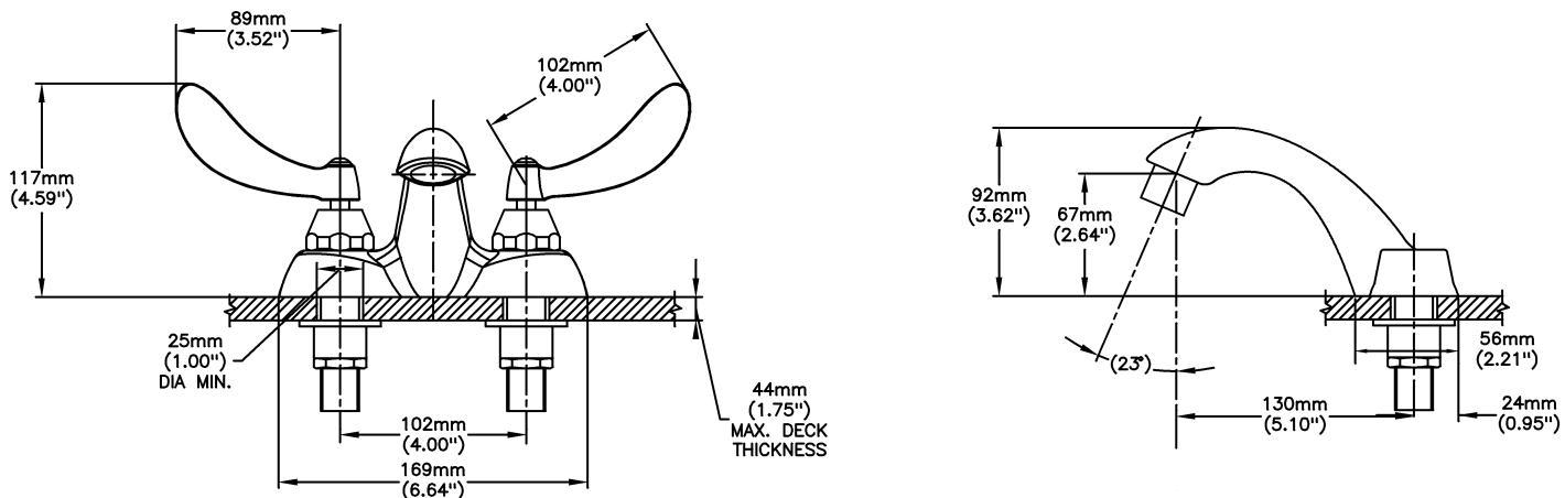
INLETS: 1/2" MIP/COUPLING NUTS (NUTS NOT SUPPLIED)
