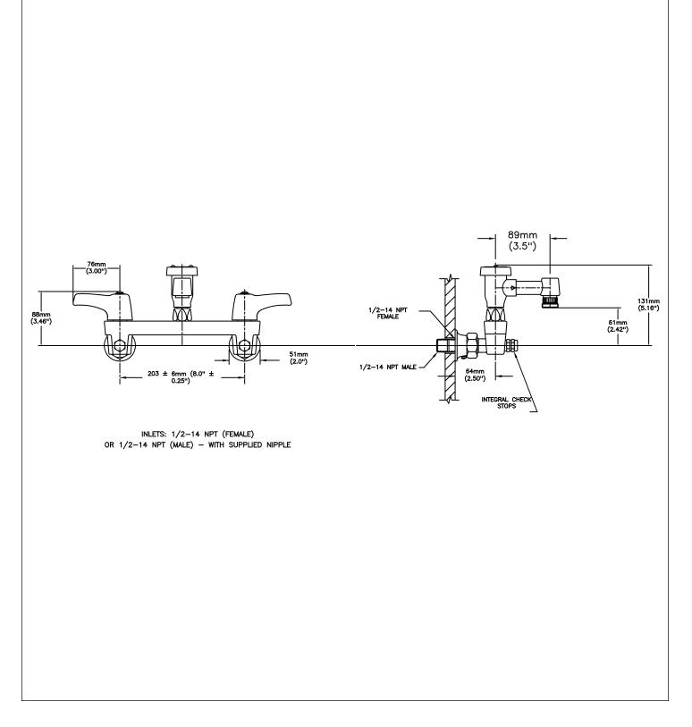
Delta reserves the right (1) to make changes to specifications and materials, and (2) to change or discontinue models, both without notice or obligation. Dimensions are for reference. Measurement may vary plus or minus 6mm(0.25"). Mounting locations are suggested only. Check with local codes for requirements in your area. This spec was produced May 04, 2021.
