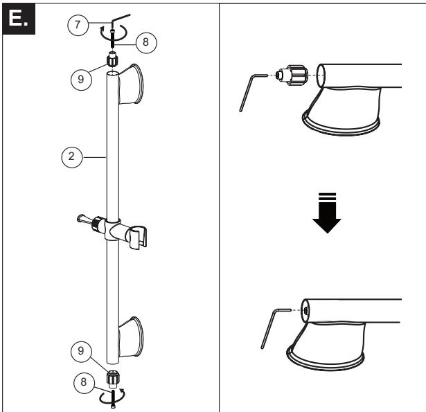
**E.** Insert an adapter (9) and screw (8) into an end of the slide bar (2). Use the included Allen wrench (7) to tighten the screw. Repeat for the other end of the slide bar.
