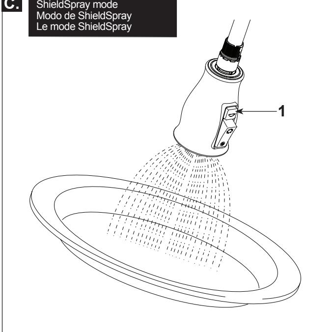
**C.** With the wand undocked, press **button 1** to use the ShieldSpray mode.
