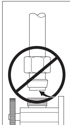
**Ensure tube is fully inserted into stop before sliding sleeve down to engage top of fitting.**
