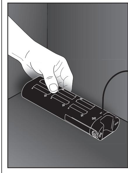
**8** Load 6 "AA" batteries as indicated on the case. For longer battery life, remove the adapter (1) and install 6 "C" batteries. **Note:** Make sure the batteries are aligned properly (+/-).
