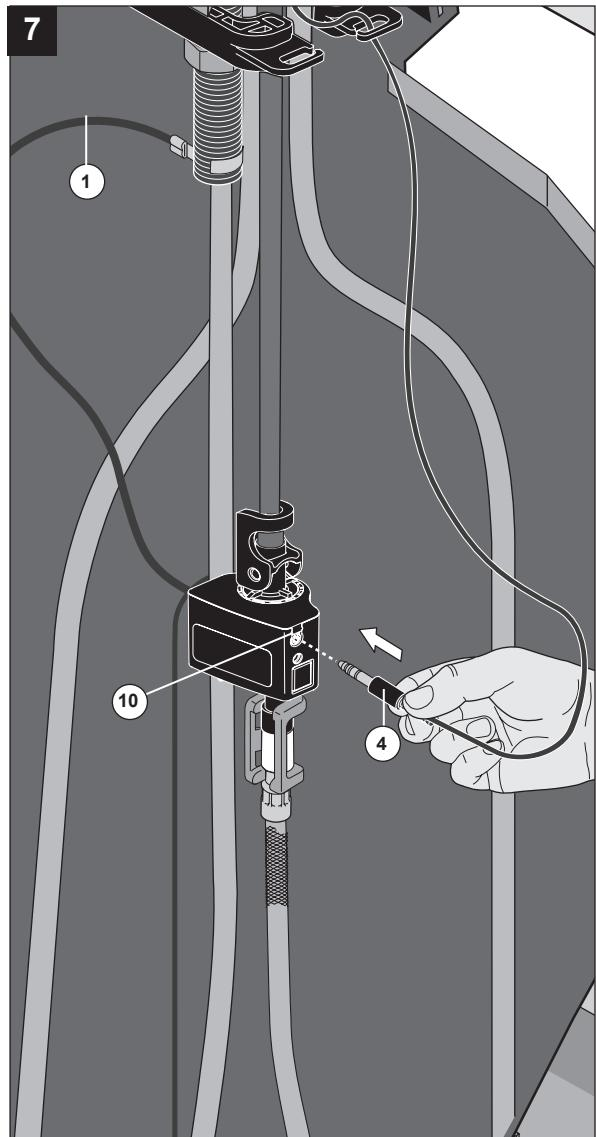
**6** Briefly touch the cold stop or other ground with hand to dissipate any static charge. **Pull-down models:** Attach wire (1), from the solenoid assembly, onto the mounting shank (2) or onto the groove on the contact nut (3). Orient clip (1) so wire exits away from wire (4). **Pull-out models:** Attach orange wire from solenoid (5) to orange wire from spout (6). **Lavatory models:** Slide wire (7) over mounting stud (8) and secure with nut (9).
