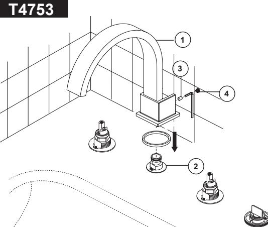
**NOTE:** The deck and valve rough-in must be finished before installing the trim kit.
