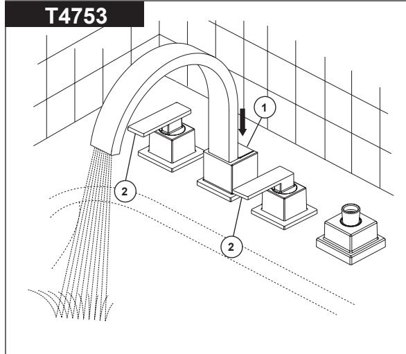
Thread stem extender (1) into valve stem (2). Install gasket (3) onto bonnet nut (4), install glide ring (5) into handle base (6), and place the base over end valve. Install handle (7) over stem extender and secure with set screw (8). Repeat for other handle. Note: If surface is uneven, use silicone sealant under the handle base.
