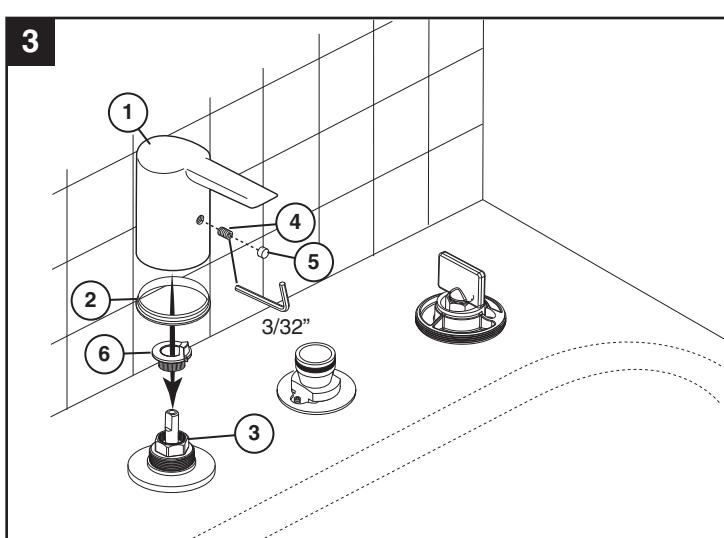
**NOTICE** If there is an orange lift rod retainer (2) in the bottom of the spout body (1), remove it prior to spout installation. To remove the retainer (2), hold spout (1) firmly over flat surface and pull up on lift rod (3). The orange retainer (2) should drop from bottom of spout. Properly dispose of retainer.
