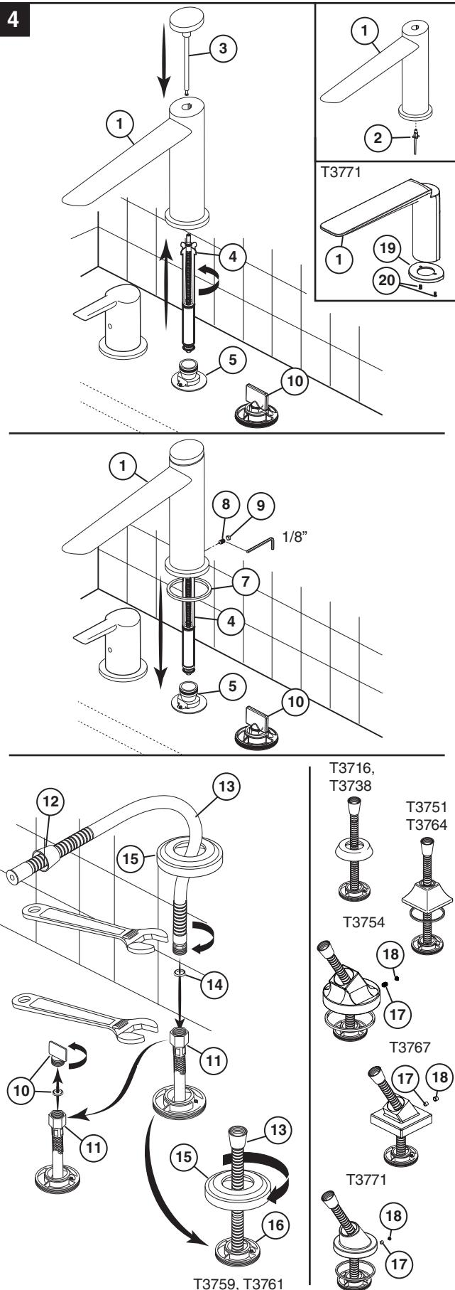
1. Remove the stream straightener and gasket (3) from the spout (5) using the wrench (4) supplied.
