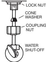
These parts must be used as illustrated to insure water-tight connection. Use of existing coupling nut may result in water leakage. Water supply tube or pipe must extend at least 1/2" (13 mm) inside threaded shank of valve (does not apply to flanged tubing).
