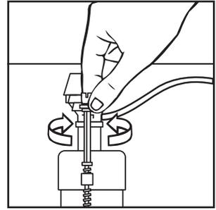
Turn on water supply. Submerge the FLOAT CUP under the water for 30 seconds. Adjust the water to desired level by turning WATER LEVEL ADJUSTMENT ROD and moving FLOAT CUP up or down.
