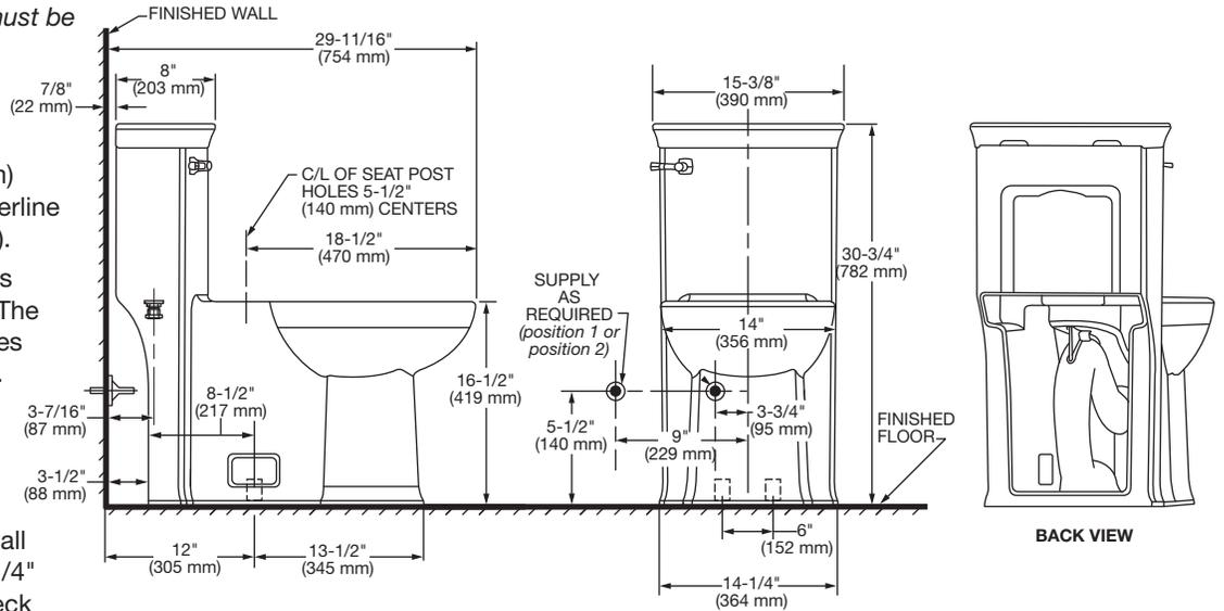
**IMPORTANT:** Water supply on the wall is required at 3-3/4" (95 mm) or 9" (299 mm) from centerline of the toilet (see rough-in).
