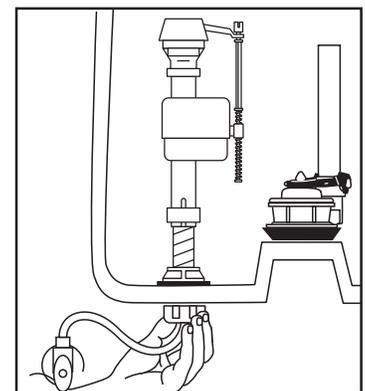
With correct washers in place (see Step 8a), tighten COUPLING NUT 1/4 turn beyond hand tight. DO NOT OVERTIGHTEN.
