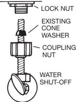
Use existing spiral cone washer. Fluidmaster cone washer may not seal completely on spiral type supply line.
