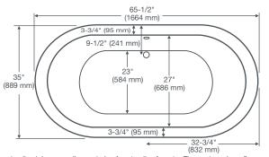
Freestanding tubs use wall-mounted or freestanding faucets. The waste and overflow assembly is concealed between the walls of the tub, eliminating the need for a decorative exposed drain kit. Dotted Line Represents Bathing Well
