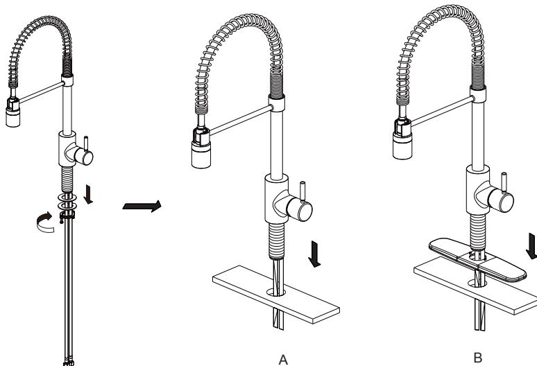
Optional deck plate (to cover existing mounting holes in the sink deck)/
