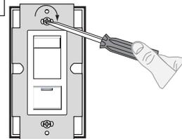
Installation may now be completed by carefully positioning all wires to provide room in wall box for control. Mount control into box with mounting screws supplied. Attach wallplate.
