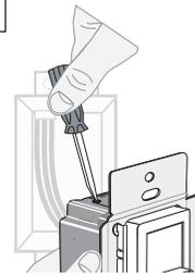
This Fan Speed Control incorporates a minimum fan speed adjustment that allows you to set the level of speed when the slider control lever is in the lowest position.
