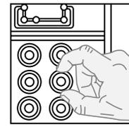
**Step 2** **Removing existing switch:** Remove existing wallplate and switch mounting screws. Carefully pull switch from wall box. **DO NOT** remove wires attached to the switch at this time.
