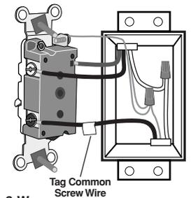
**3-Way:** Look at the back of your switch. If there are 3 wires connected to three screw terminals (not including a green or bare copper wire used for grounding), you have a 3-Way switch. Note that one of the screw terminals will usually be a different color (black) or labeled Common. Tag that wire with electrical tape to identify.
