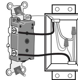
**Single-Pole:** Look at the back of your switch. If there are 2 wires connected to two screw terminals (not including a green or bare copper wire used for grounding), you have a Single-Pole switch.
