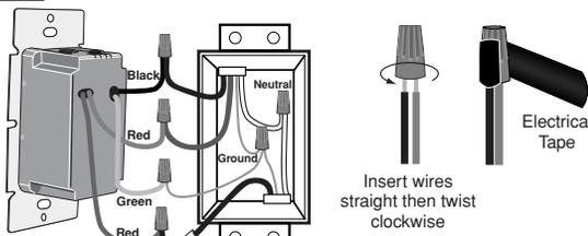
Fan Speed Control 3-Way Switch Common Terminal (Black Screw)
